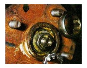
When removed, you will see the small rollers that the entire weight of your car sits on! Give everything a generous dose of molybdenum disulphide grease and work it in to the moving parts of the bearing.
